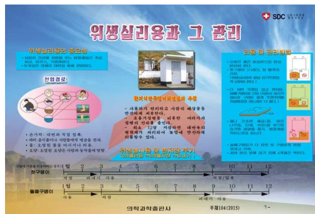
Hygiene promotion poster explaining the use and advantage of double pit latrine)
