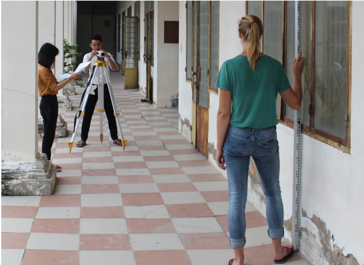
Figure 3: Levelling with a theodolite in Long Xuyen in the Mekong Delta by GIZ for measuring land subsidence at buildings (photo credit: Kim de Wit)
