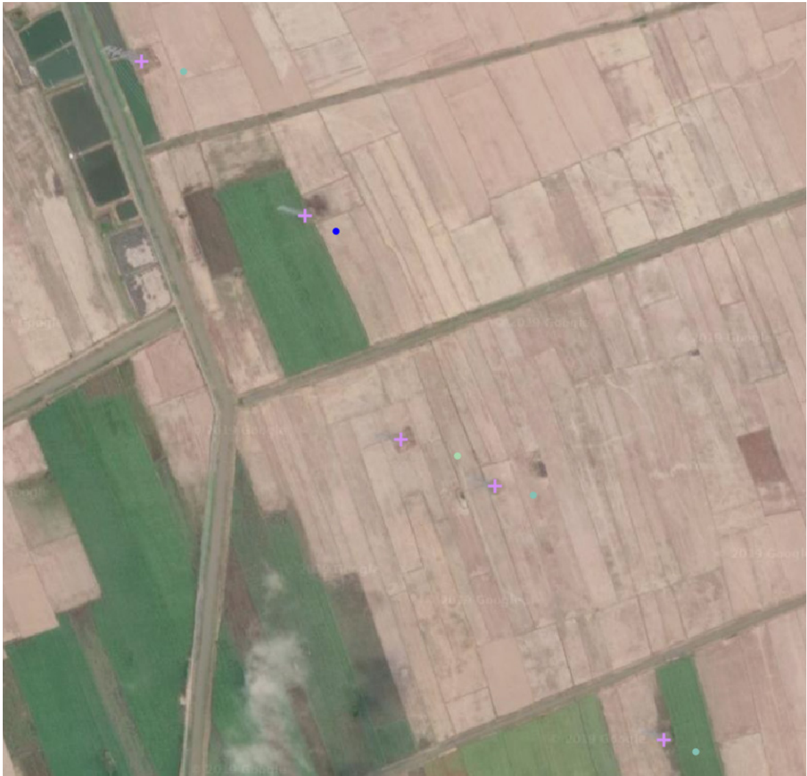
Figure 14: Centre of the foundation of pylons marked with crosses, PSI with coloured dots. The distances are between 40 to 50m.
