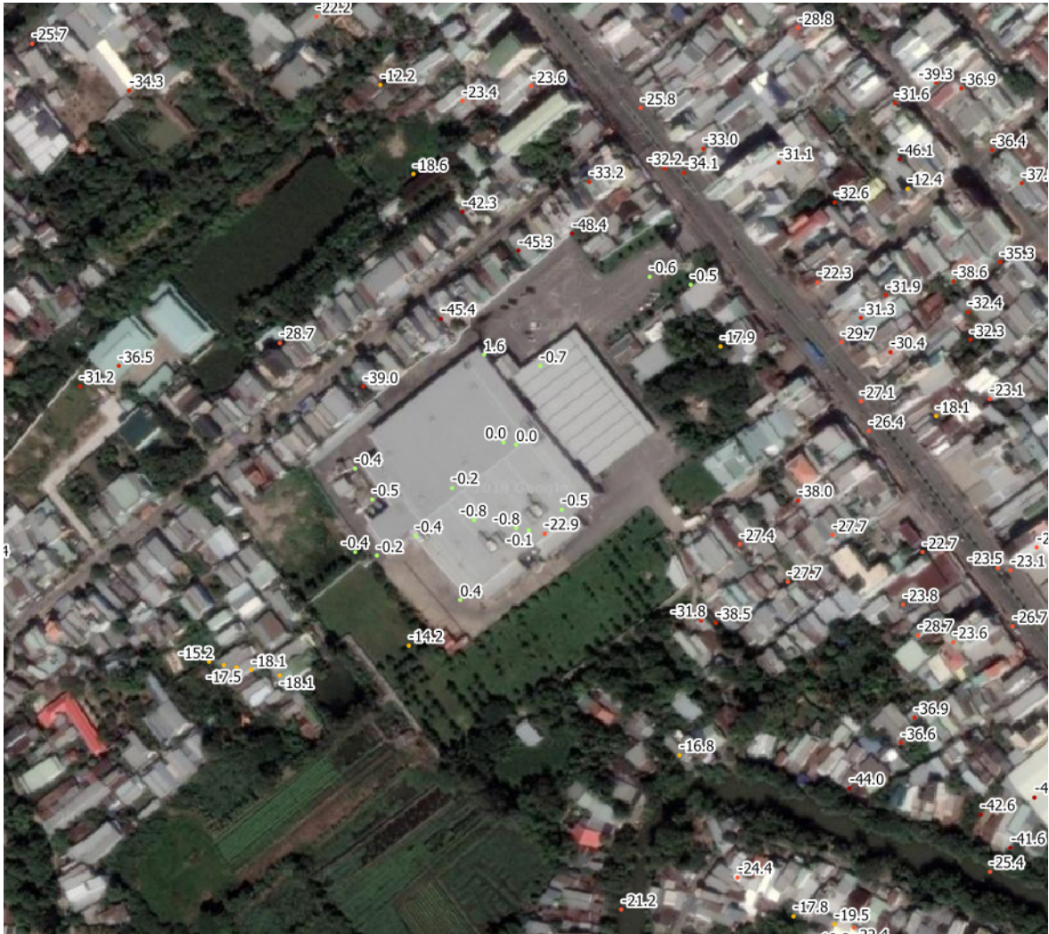
Figure 16: Average vertical velocity in mm per year 37 , displayed on Google Earth image as background.
