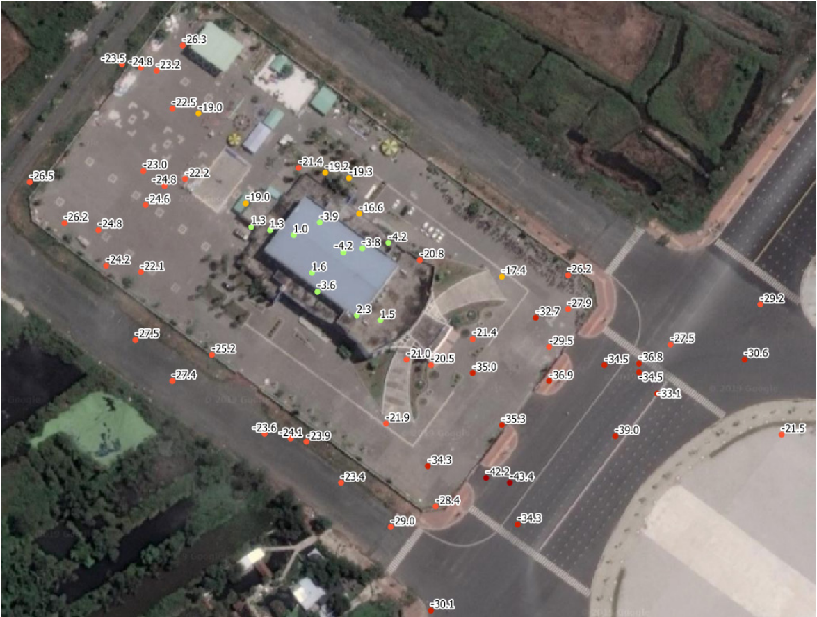
Figure 15: Average vertical velocity in mm per year -36 , displayed on Google Earth image as background.
