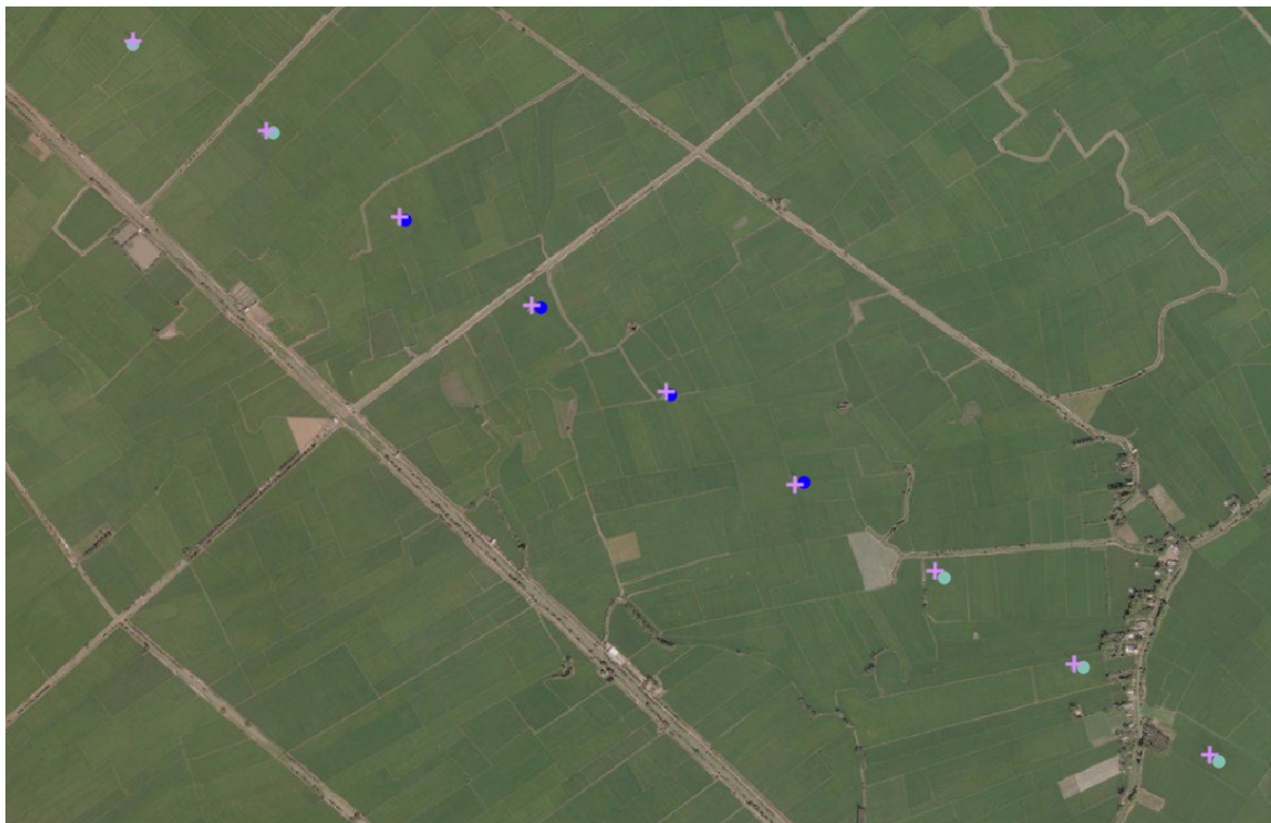
Figure 13: Power pylons marked with pink crosses and PS (circles with colours according to vertical velocity) displayed on Google Earth image as background.
