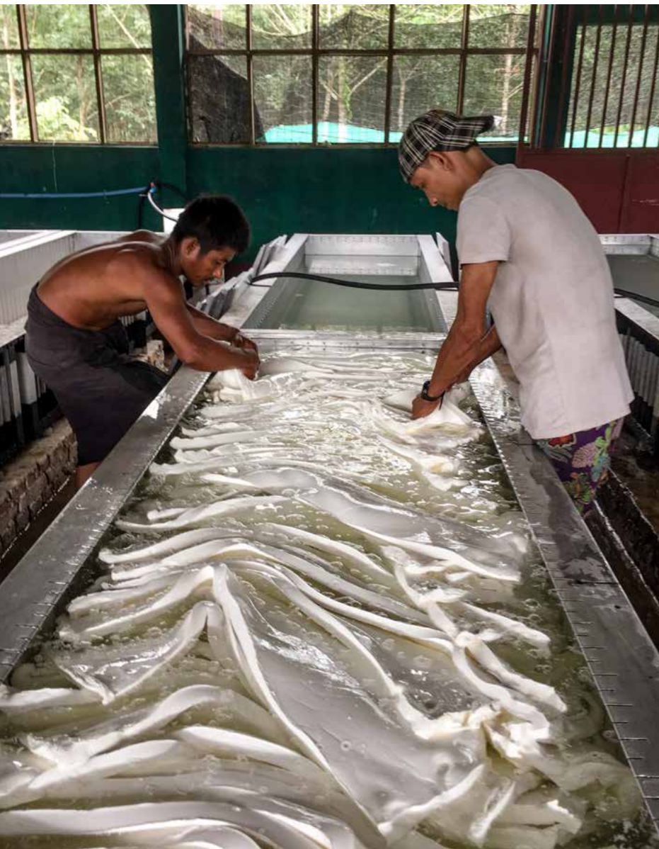
Latex sheets ready for the smoke house, © Markus Buerli / Embassy of Switzerland in Myanmar
