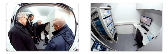
**Measuring car:** the car measures the concentration of PM10 particulate matter, which requires special attention in the autumnwinter period due to adverse meteorological conditions. Moreover, it provides information about pollutant gases in the air and allows samples to be taken for further laboratory tests.
