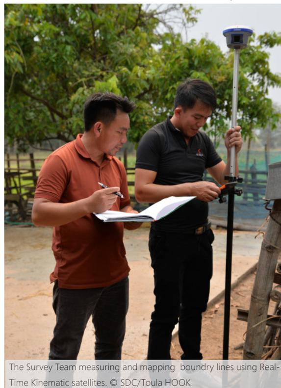
The Survey Team measuring and mapping boundary lines using Real-Time Kinematic satellites. © SDC/Toula HOOK
