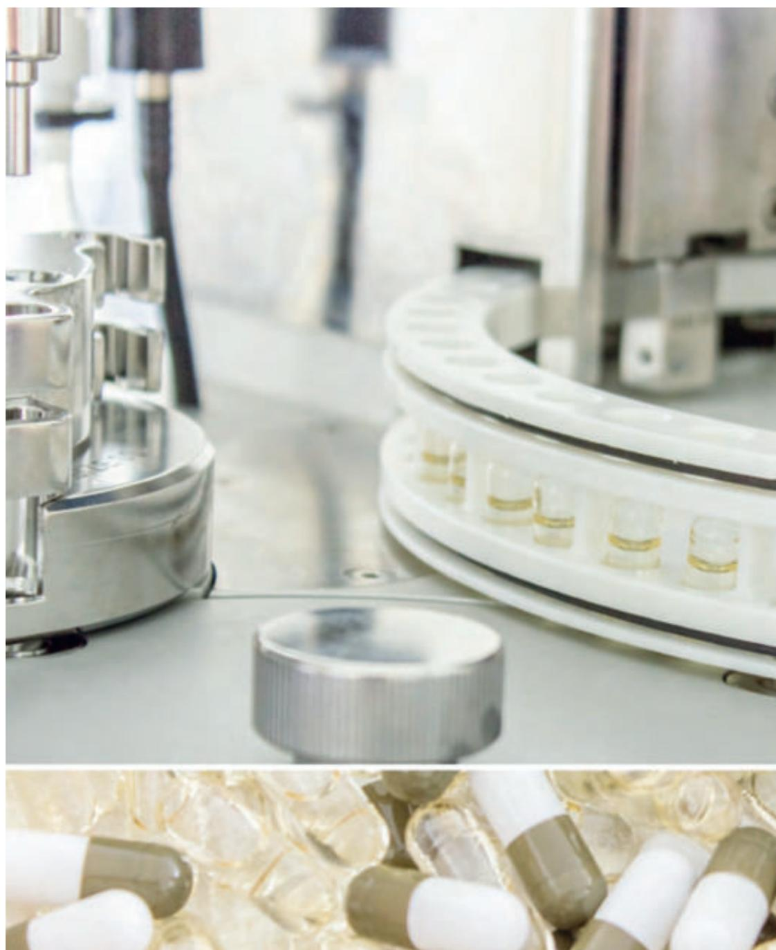
Desktop manufacturing for the novel liquid capsule dosage form of a Pheroid®-containing product now commercially available.
