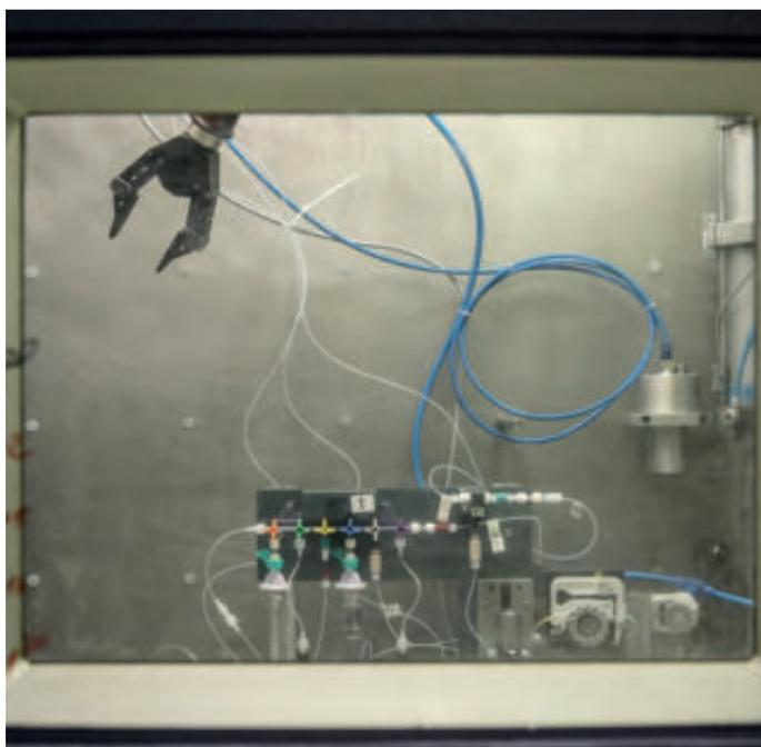
*Chemical separation system for Tb radionuclides.*
