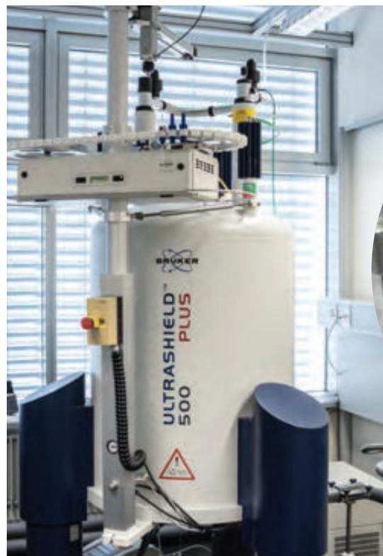
Microprobe NMR instrument for structure analysis.
