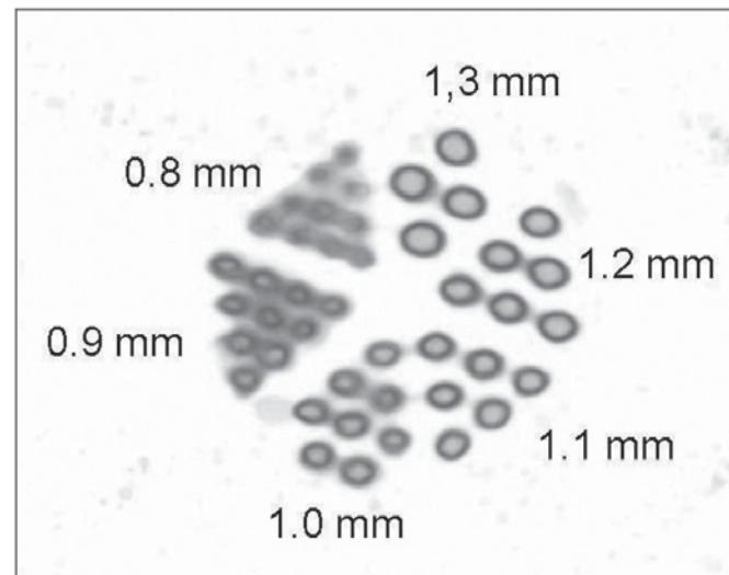
Derenzo phantom filled with Tb-155 solution. Pinhole diameter range from 0.8 mm to 1.3 mm.
