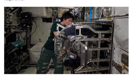
ESA astronaut Samantha Cristoforetti preparing the BIOLAB research facility for the TripleLux-B experiments on board the ISS Columbus module. The TripleLux experiments were developed by the Universities of Zurich and Berlin to study immune system responses in muscle cells. Implementation on board the ISS was planned and supported by the Swiss USOC in Hergiswil. © ESA
