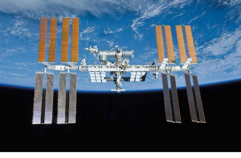
The International Space Station in orbit, photographed from a space shuttle after it undocked in May 2010. The pressurised modules are clearly visible in the middle, and so is the large horizontal truss on which the great wings bearing the solar panels are mounted. A Soyuz spacecraft is visible at one of the zenith port on the station. The European research module Columbus is attached to the starboard side of the station.  $\circ$  NASA
