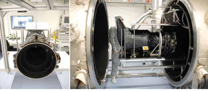
CHEOPS's structural and thermal model (STM) in the laboratory at the University of Bern. Left: Front view shows the baffle entry and radiator ensuring thermal control of the instrument. Right: the instrument is being placed in the thermal vacuum chamber for environmental tests.  $_{\rm CHEOPS\,Team\,/\,University\,of\,Bern}$
