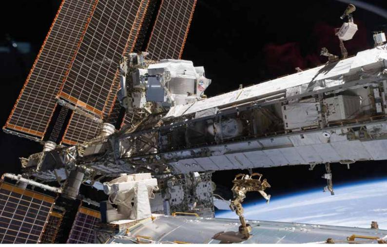
The Alpha Magnetic Spectrometer, installed on the truss section of the International Space Station  ${\tt o}$  NASA
