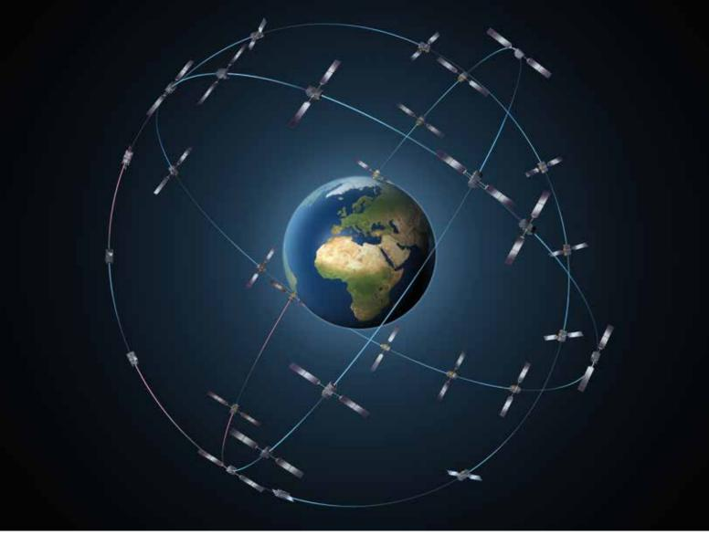
The complete Galileo constellation with eight satellites in each of three orbital planes (plus two reserve satellites in each orbital plane).  $\odot$  ESA
