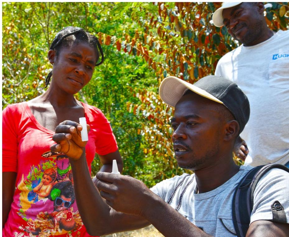
Testing the water's chlorine content
